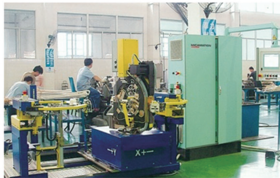
从瑞士引进的自动包带机 Automatic taping machine introduced from Swiss
