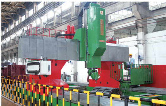
XHZ2925-10 定梁动柱式龙门加工中心 XHZ2925-10 fixed-beam and moving-column gantry machining center CNC
