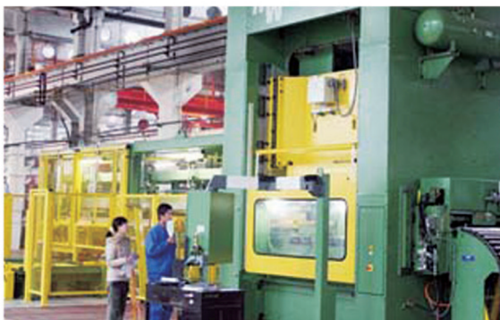
4000KN 双点闭式冲压机自动生产线(德国) Automatic production line for 4000kN dual-point closed punching machine (Germany)
