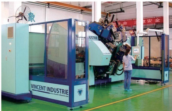
从法国引进的线圈自动涨型机 Automatic coil expansion machine introduced from France
